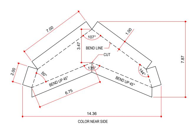
NOTES: BUYOUT **AVAILABLE COLORS** 1) USE FOR SLOPES FROM 4 1/2:12 TO 5 1/2:12 PW 2) PEAK PLATE IS USED IN CONJUNCTION WITH THE PRESS BROKE RIDGE TRIM AND METAL PEAK BOXES. 3) SUPPLIED IN PW ONLY TO MATCH PRE-FABRICATED METAL PEAK BOXES.
