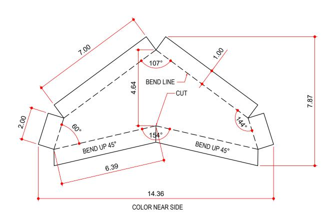
NOTES: BUYOUT **AVAILABLE COLORS** 1) USE FOR SLOPES FROM 2 1/2:12 TO 3 1/2:12 PW 2) PEAK PLATE IS USED IN CONJUNCTION WITH THE PRESS BROKE RIDGE TRIM AND METAL PEAK BOXES. 3) SUPPLIED IN PW ONLY TO MATCH PRE-FABRICATED METAL PEAK BOXES.
